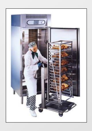
A blast chiller employs forced air in a cabinet type freezer. Utilizing wheel-in carts, food in steam table pans or packed in casings are loaded onto the shelves of the cart. The cart is wheeled into the cabinet. Hot foods are then rapidly brought through the Danger Zone (from above  $135^{\circ}F / 57^{\circ}C$  to below  $41^{\circ}F/5^{\circ}C$ ).
