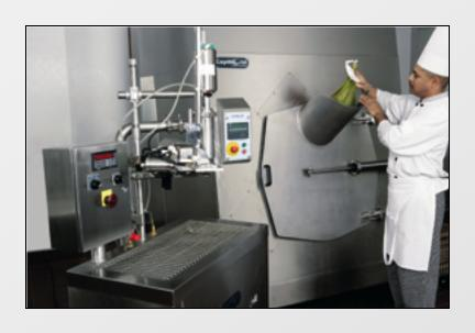
Filled casings are loaded directly into the product chiller and gently tumble circulating cold water. The tumbling action quickly removes heat from the food casings, dropping the product temperature from 180°F (82°C) to 41°F (5°C) in 60 minutes or less.
