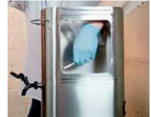
4. Place liner in urn. Feed tube through faucet opening until tube protrudes.
