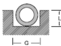
Flexi-Shield mounted in standard O-ring groove.
