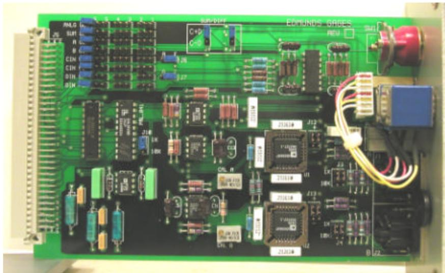
Figure 4.6a - LVDT Module E8302, current version
