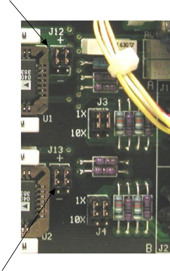
Input B Polarity Jumper
