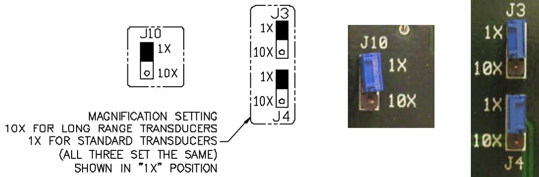
Figure 4.10 - Attenuation Jumpers, obsolete version
