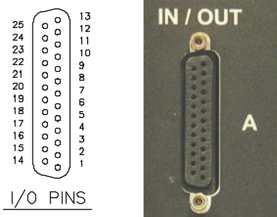
Figure 2.4 - I/O Pins
