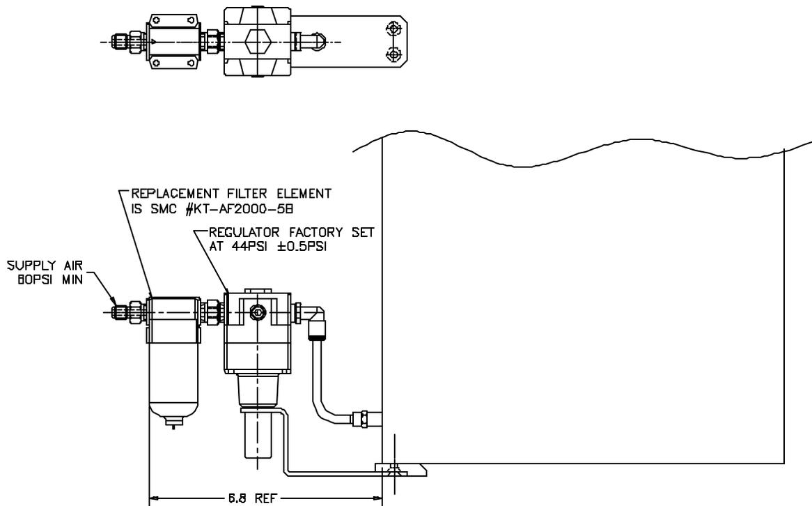
Figure 2.9 - Supply Air Filter/Regulator
