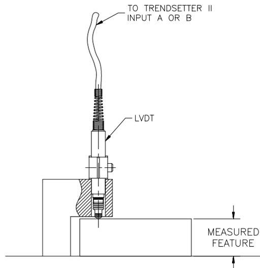
Figure 3.4 - Single Probe Application
