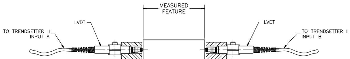
Figure 3.5 - Two Probes Application
