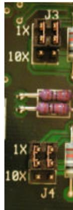
Figure 4.10a - Attenuation Jumpers, current revision
