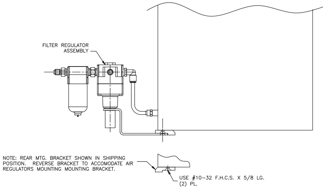
Figure 3.2 - Filter/Regulator Mounting
