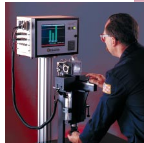
One board does it all. Edmunds universal 4-channel signal conditioning board can accommodate Edmunds LVDTs and air-to-electronic inputs with full range choices.
