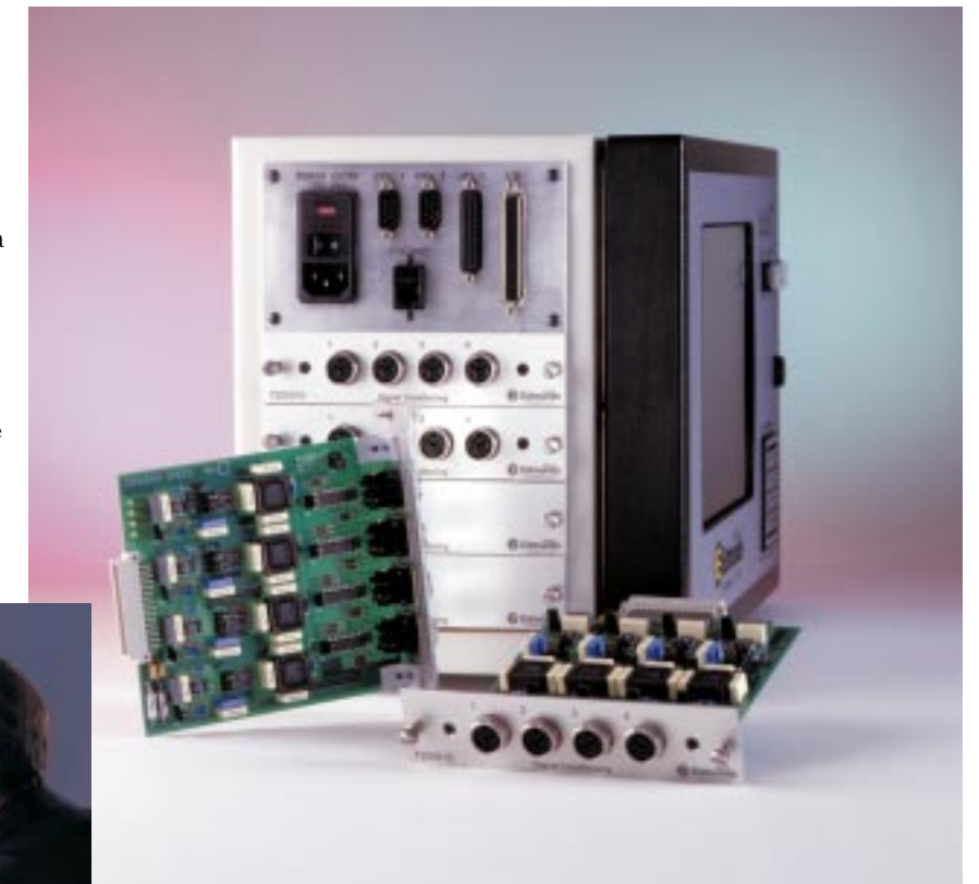
One board does it all. Edmunds universal 4-channel signal conditioning board can accommodate Edmunds LVDTs and air-to-electronic inputs with full range choices.
