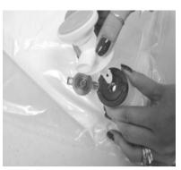
Step 2 – Take one of the dispensing valves (2 provided with each case). Placing the bag on a flat surface, push the dispensing valve firmly in as far as it will go. Now the bag is ready to install into the machine
