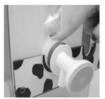
Step 7 – Continue to slide spout until it rests at bottom of channel. Repeat steps 1-7 for each bag.
