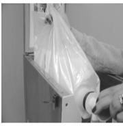
Step 5 – Grasp top of bag. Place bag into chamber while guiding spout into front channel guide.
