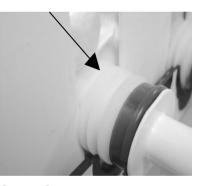
Step 6 – Slide inner spot ring (see arrow) into channel guide. Use ring closest to bag.
