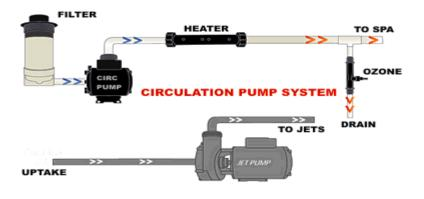
you still have the other one however a spa needs both pumps to function so it doesn't make much difference. With a 2-speed pump you have the advantage of having the normal strong massage intensity from the jets as well as the very soft intensity when the low speed is on. With a circulation pump, on the other hand, you have a few more
