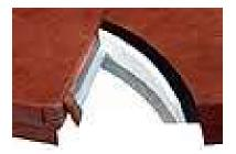
and non-cotton backing. The styrofoam should be a minimum of 9 cm. thick tapered to 8 cm for water run-off, be re-enforced at the center fold and the cover should have an efficient method of locking it against weather and curious children. Always remove the entire cover before climbing into the spa, replacing it when finished. Most dealers also offer special cover "lifters" so that one person can remove
