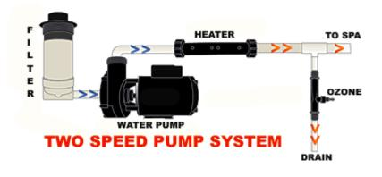
speed is used for massage and this means that all the water returning into the spa is always coming out of all of the massage jets.
