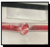
Image 3 Actual burst on detection tubing
