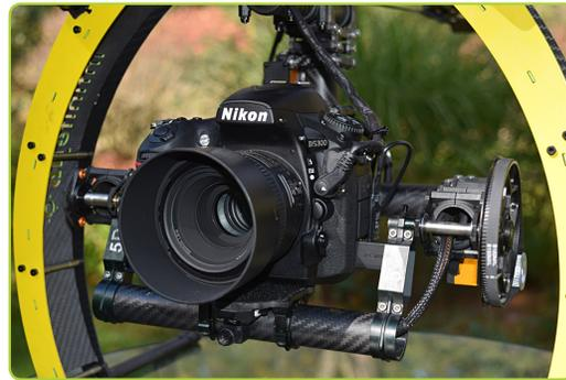
The standard Surveyor 630 UAS includes a Nikon D5300 DSLR outfitted with a 28mm prime lens and GPS.
