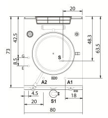
KEY E power supply G gas connection H2O water inlet S water outlet
