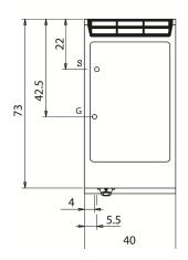
KEY **E** power supply **G** gas connection H2O water inlet **S** water outlet
