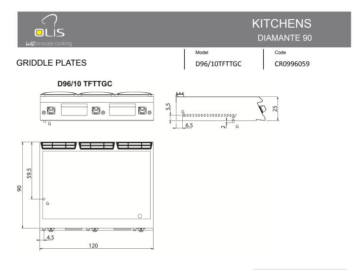
KEY E power supply G gas connection H2O water inlet S water outlet
