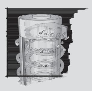
Ice evaporator with stainless steel auger
