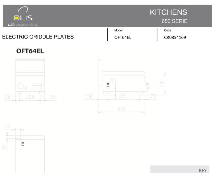
E power supply G gas connection H2O water inlet S water outlet
