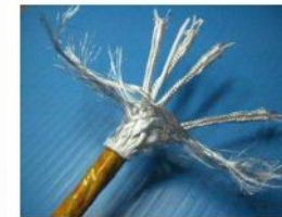
Low Mass SpaceWire Cable AWG28: 43g/m
