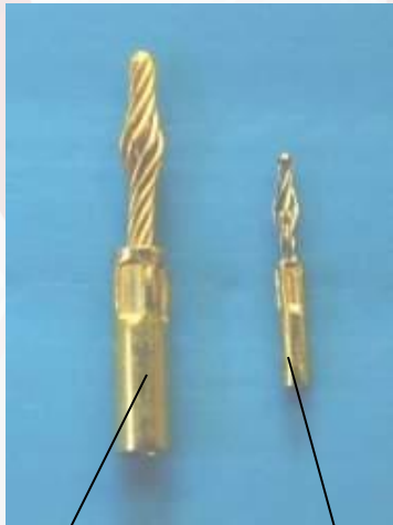
Micro D NanoD Twist Pin contacts
