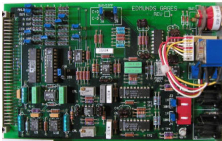
Figure 4.6 - LVDT Module E8302, original version
