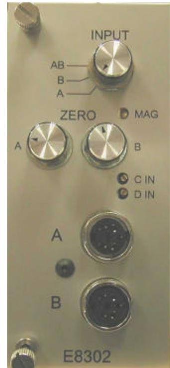
Figure 2.7 - E8302 (2) Channel LVDT Signal Conditioning Module
