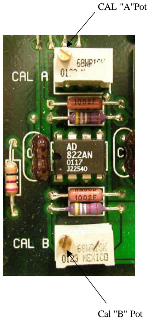
Figure 4.11 - Cal "A" and "B" Potentiometers
