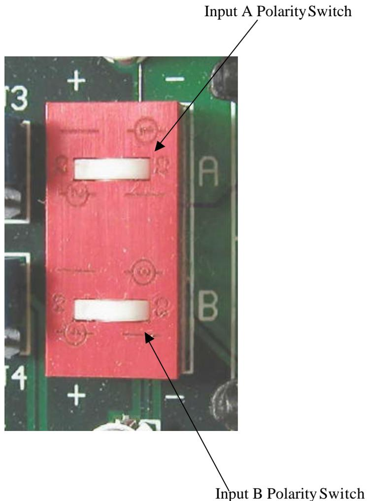
Figure 4.7 - Polarity Switch, original version
