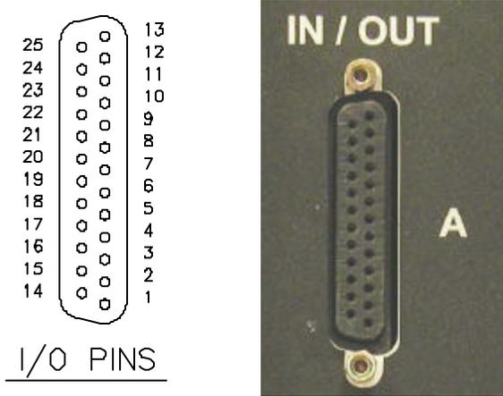
Figure 2.4 - I/O Pins
