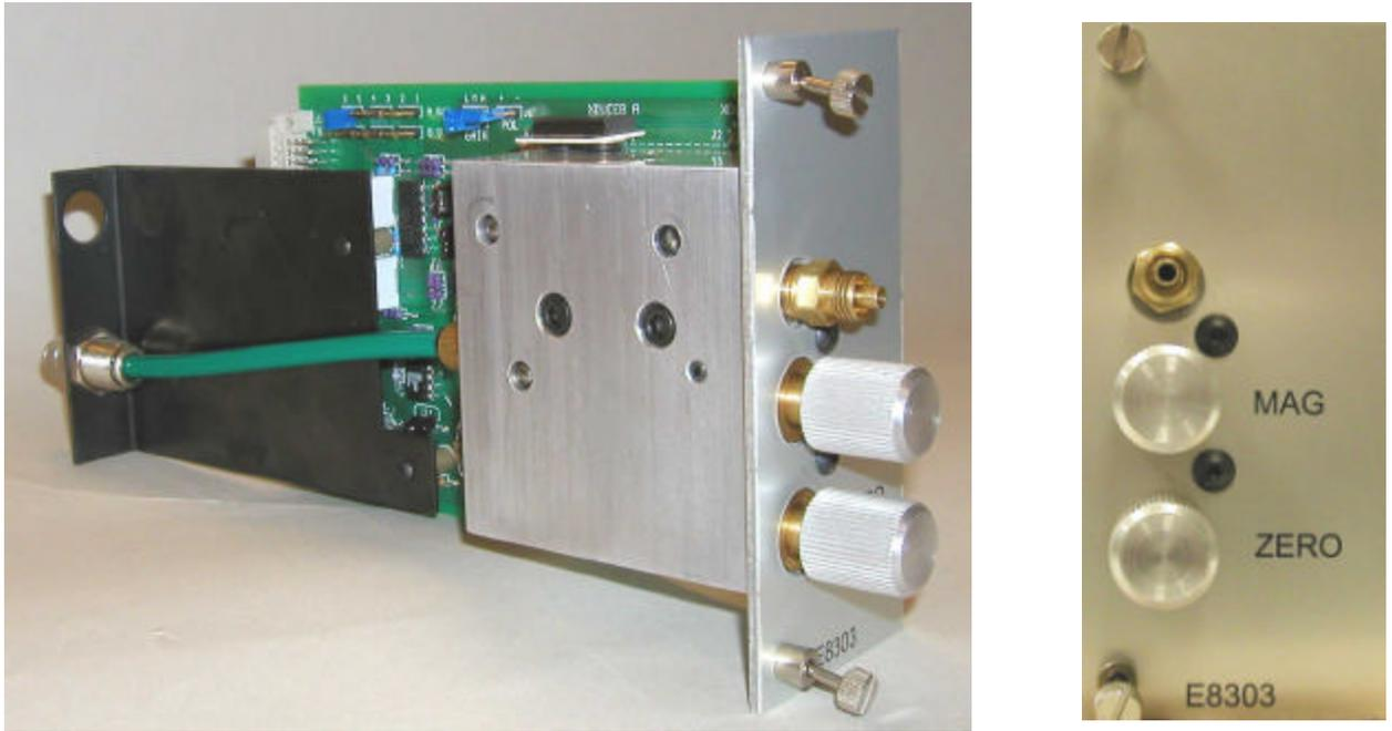
Figure 2.8 - E8303 (1) Channel AE Signal Conditioning Module
