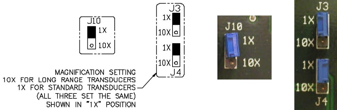
Figure 4.10 - Attenuation Jumpers, obsolete version
