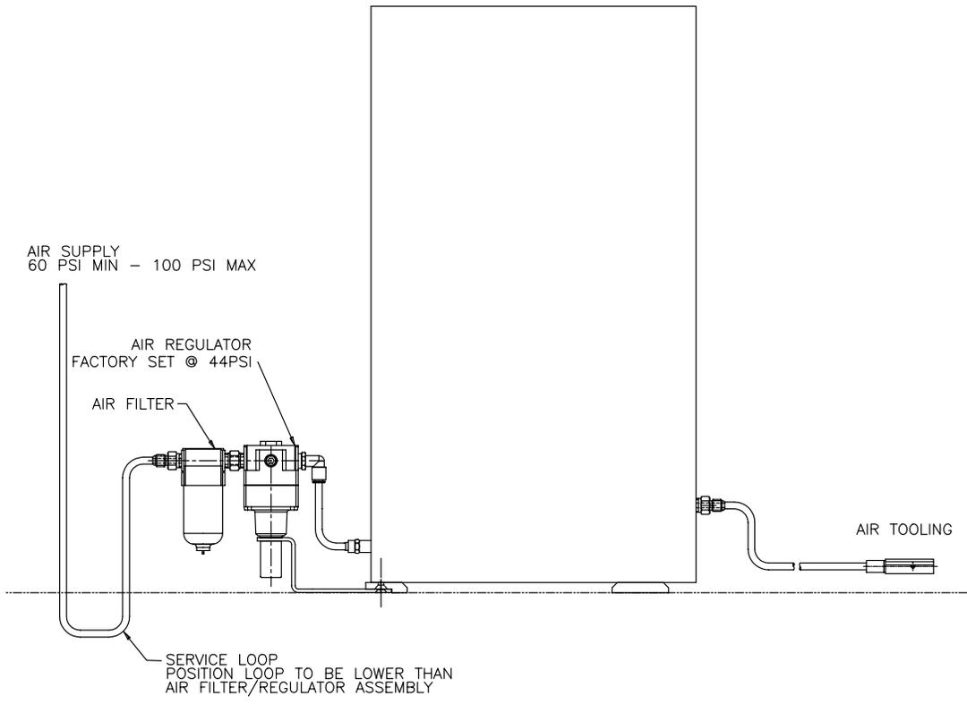
Figure 3.3 - Air Connections
