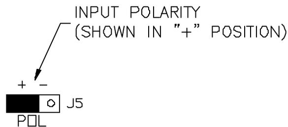
Figure 4.3 - Polarity Jumper
