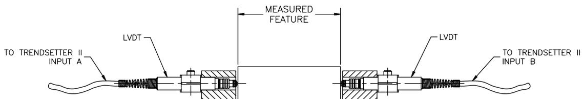
Figure 3.5 - Two Probes Application
