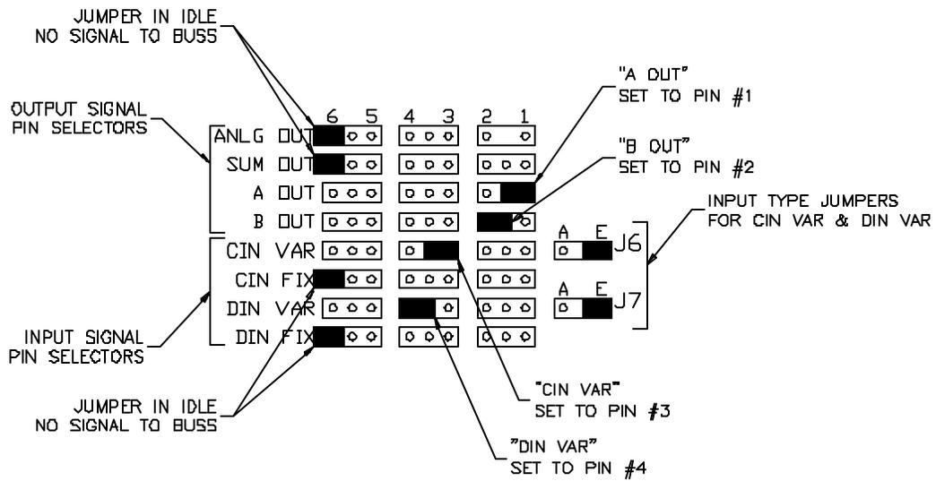
Figure 4.8 - Input/Output Jumpers
