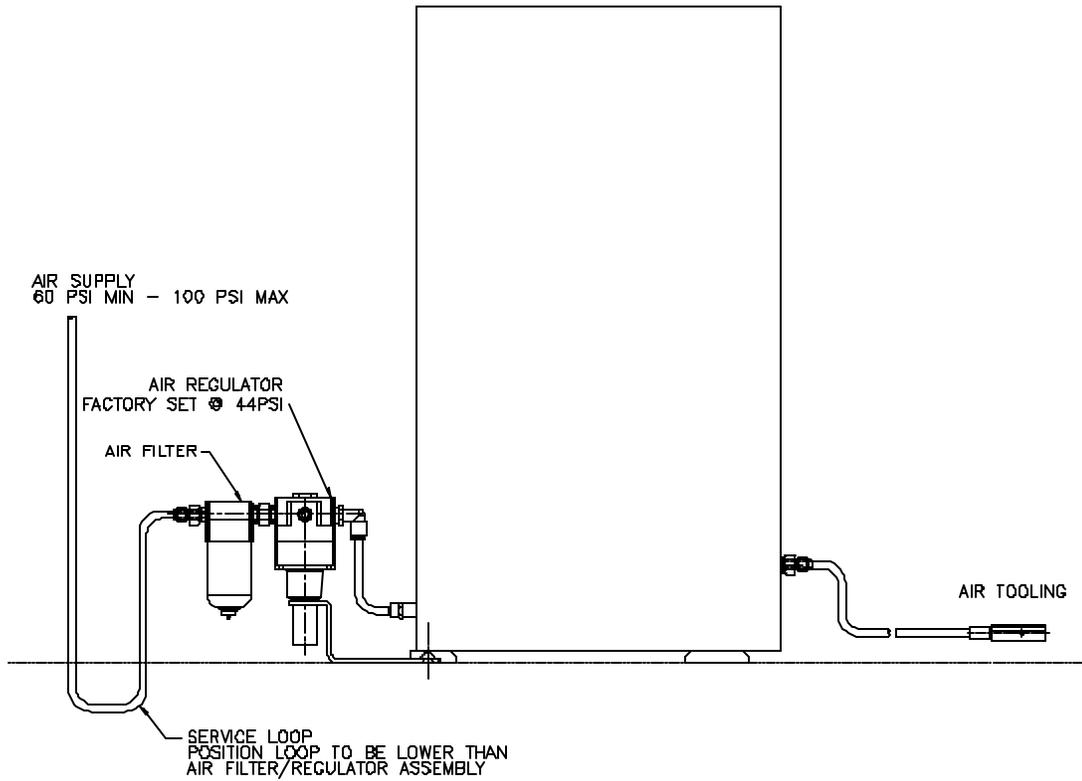
Figure 3.3 - Air Connections
