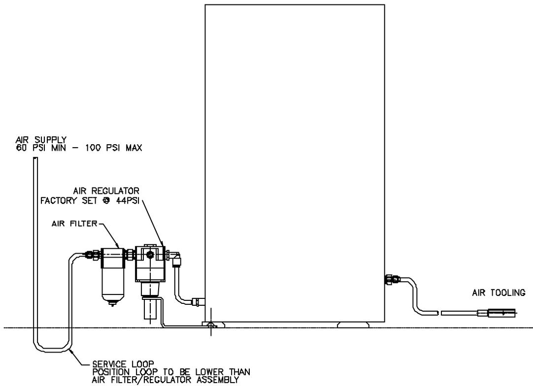
Figure 3.3 - Air Connections
