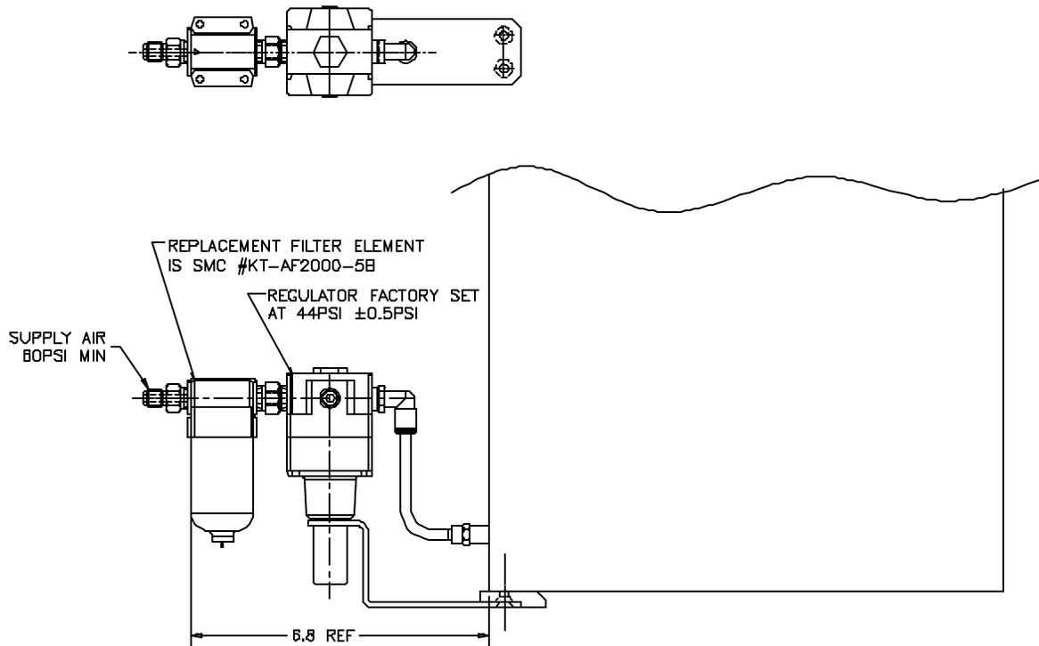
Figure 2.11 - Supply Air Filter/Regulator
