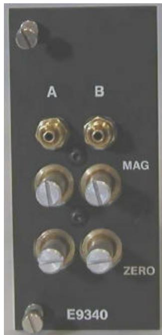
Figure 2.10 - E9340 (2) Channel AE Signal Conditioning Module
