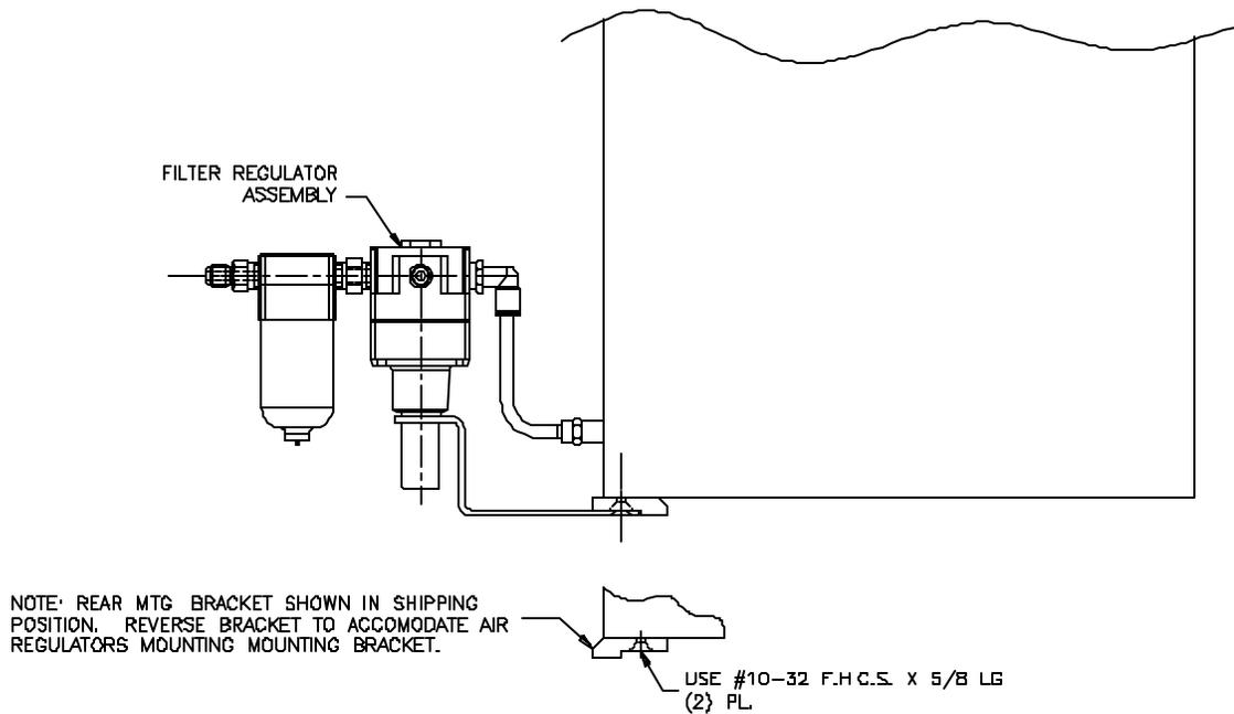
Figure 3.2 - Filter/Regulator Mounting
