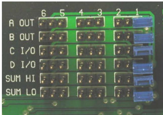
Figure 4.5 - Input/Output Jumpers
