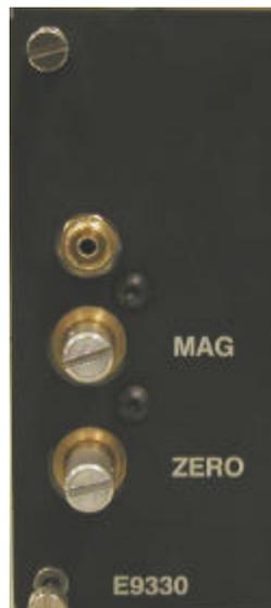
Figure 2.9 - E9330 (1) Channel AE Signal Conditioning Module
