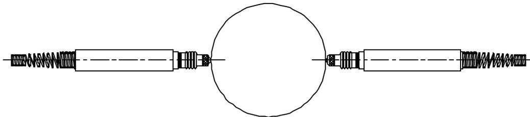
Next, we must apply a multiplier to the probes outputs that is dependant on the application. The multiplier is determined by the number of probes used to perform the measurement or to correct any ratio that may be introduced by any contact arms or tooling.
