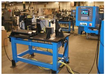
Fabrication of welded axle tubes rely upon the accurate location of the part in the automated welding application and subsequent machining operation of the critical dimensions. The same robots used in the welding process can easily load and unload a machine tool and or gaging station to close the loop on a completely automated cell.
