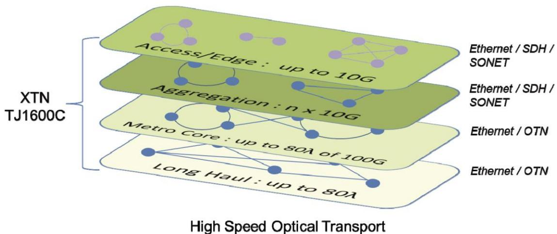
**ELEMENTOS***CAMADA ÓPTICA DWDM / CWDM*
