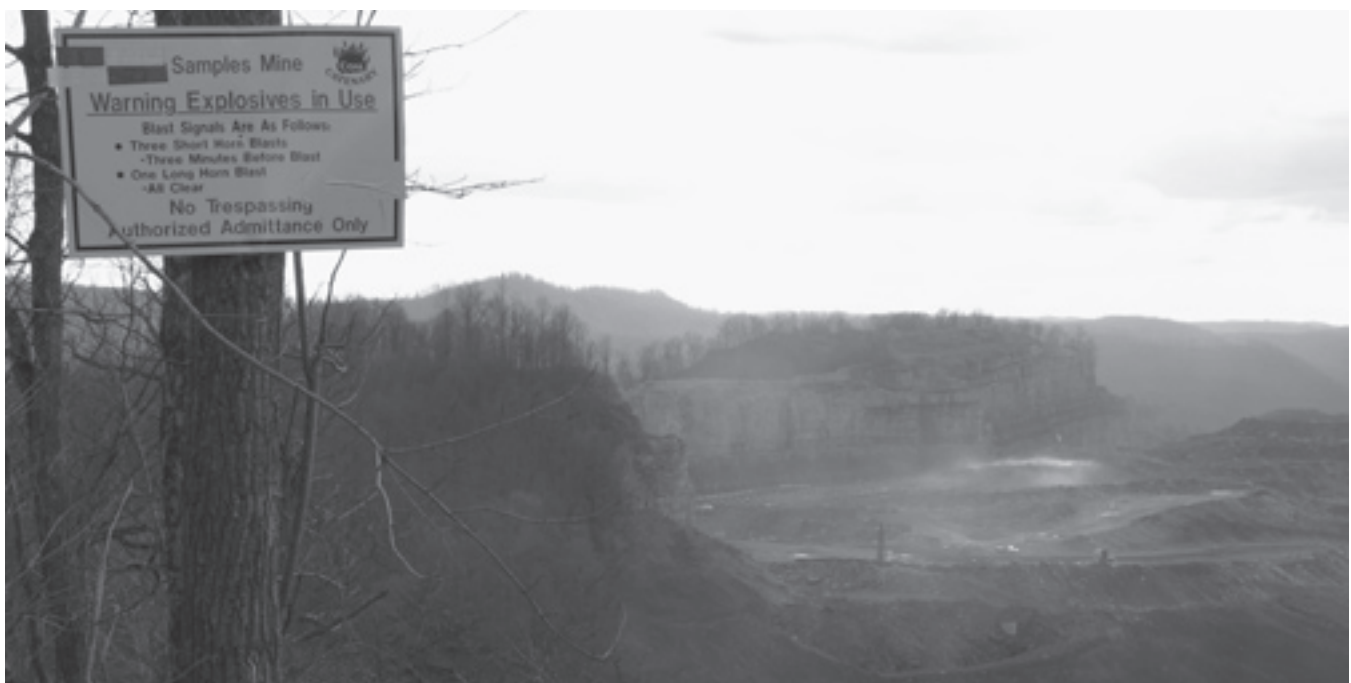
Another view of mining on Kayford Mountain. The “explosives” referred to on the sign are used to loosen rock and topsoil.
