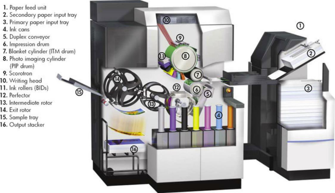
Figure 3: Indigo industrial LEP technology printer – main units [10].
