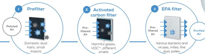
Function principle of the air purifier: Domestic dust, animal hairs, smells, pollen, harmful gases and various bacteria and viruses are filtered out of the air using a triple-layer filter system.
