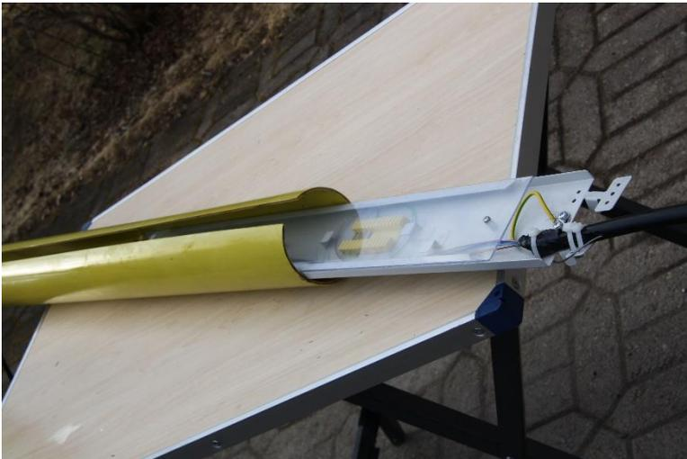
Bring up the split cable tube with a smaller splitting groove and direct the cable or cables to this groove. Pull the tube over the splice tray so that the splice tray enters the center of the tube.
