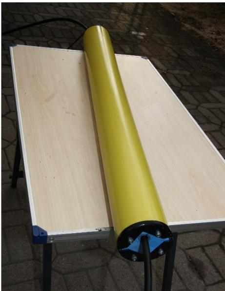
Press the remaining split cable tube on to protect the extension. Position the top tube so that its slit comes to the opposite side to the slit of the inner tube.
