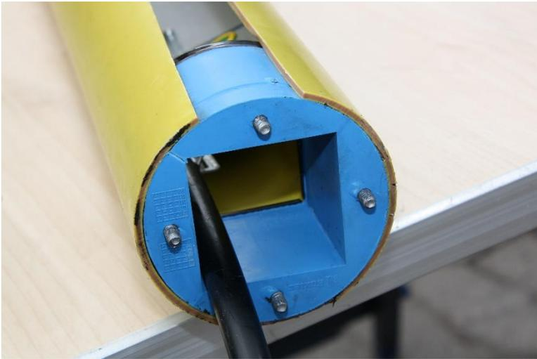
Push pass-through frames to the ends of the tube.
