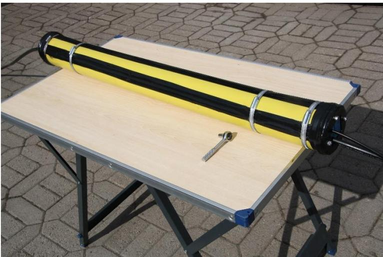
Open the hose clamps that come with the package and install them on top of the joint closure. Install two hose clamps at the ends of the joint closure and the other two quite close to the ends of the joint closure.
