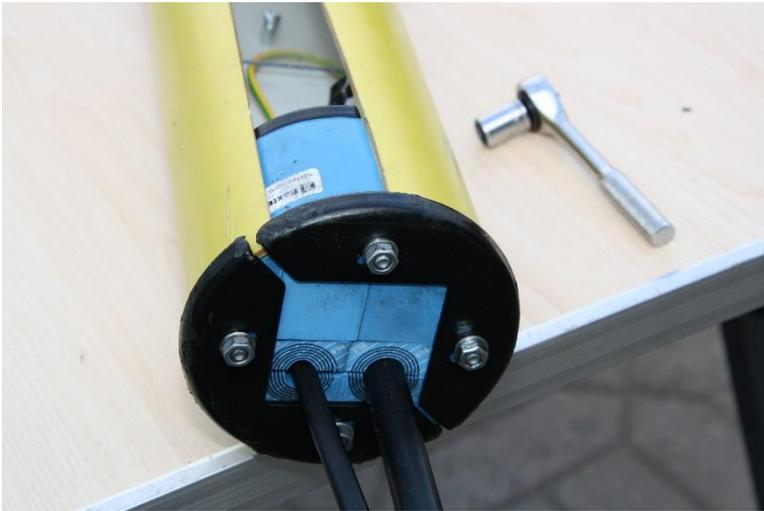
Attach the metal supports of the pass-through frame but leave the nuts loose.
