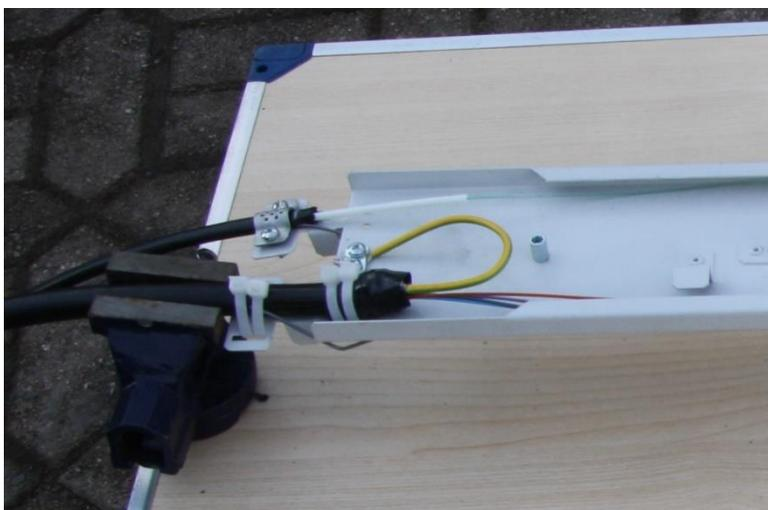
Cables attached and their metal parts connected to the splice tray.
