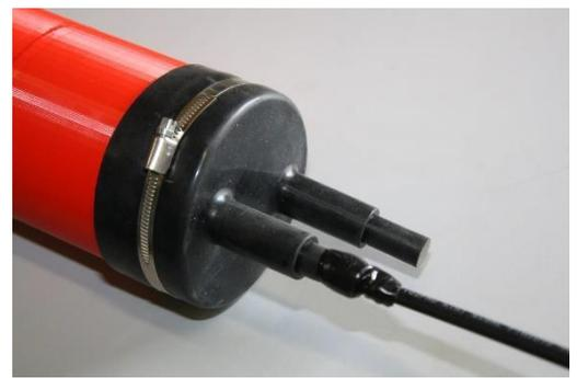
Cable gland sealed with PVC-surfaced vulcanized tape.
