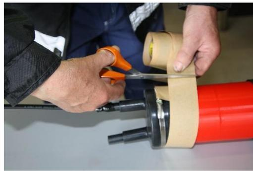
The tape is rotated with the protective paper a turn around the housing, leaving a small overlap and cutting the required length.
