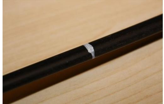
Mark the place for grounding to one of the cables coming into the joint closure with steel traction elements.
