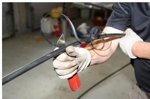
Peel the sheath off the steel wires along the entire length to be peeled.
