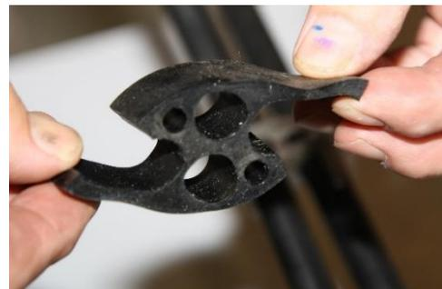
Split the sealing piece of the cable gland with a sharp knife
