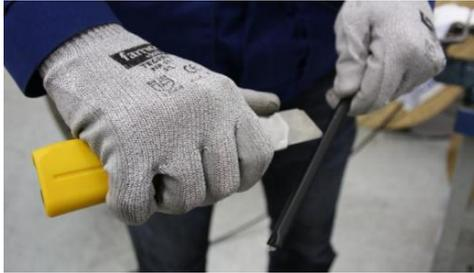
Split the sheath from the end of the cable from the grooves of the strength members for about 15 cm.
