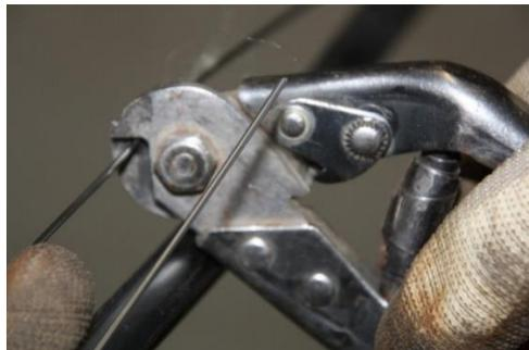
Cut the steel wires at each end to a length of about 20 cm.
