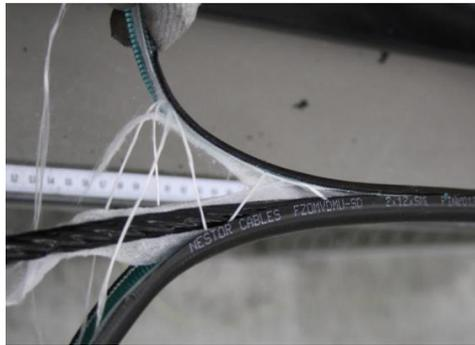
Pull the sheath open to the starting point of the peeling.
