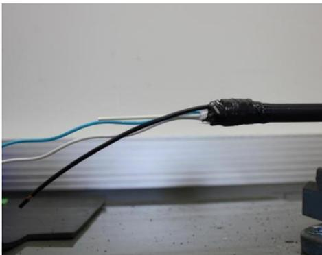
Protect the connector of the grounding wire with insulation tape. After that squeeze the sheath halves against each other and tape them together
