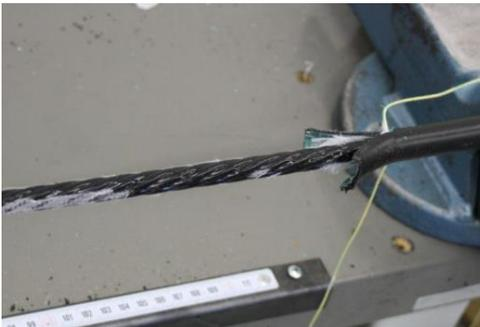
Cut the halves of the sheaths to about 3 cm in length and remove the white swelling strip and its binding threads from the middle sheath. Also cut the tear wires at the base of their splitting grooves.
