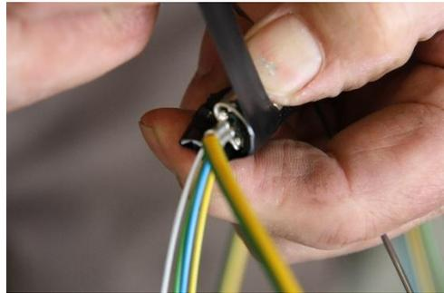
Protect the connector of the grounding wire with insulation tape.
