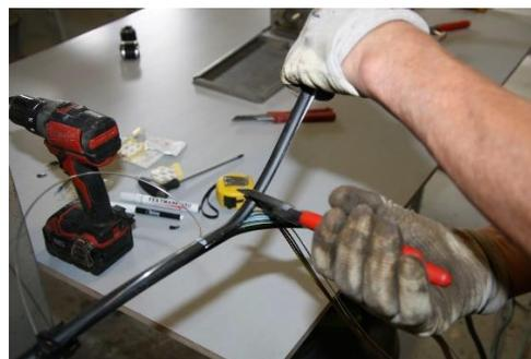
Cut off the halves of the sheath so that the remaining pieces are about 3 cm long.
