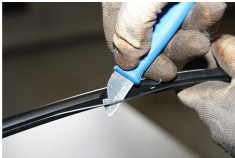
Dig out the steel wires.
