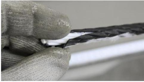
Open up the middle sheath from the end with a knife, enough to get a grip from the edges.
