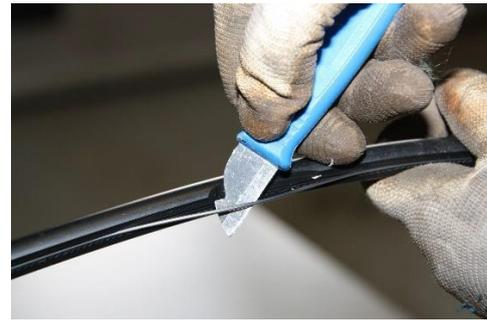
Dig out the steel wires.
