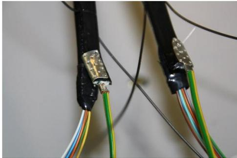
The connectors of grounding wires installed into FZVD2PMU Flex direct buried cables. Notice the protection of fiber tubes against one of the halves of the cable sheath.
