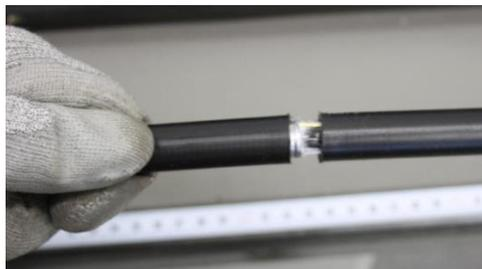
Pull the severed part off the middle sheath to get the yellow tear wires out.
