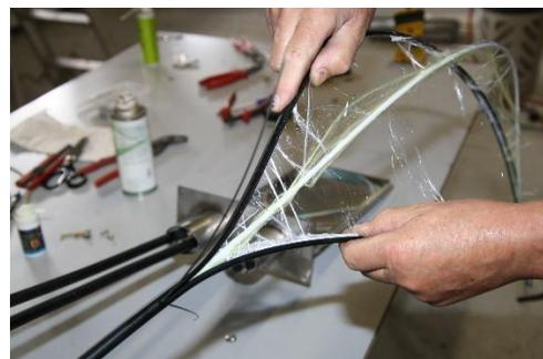
Bend the cable slightly to separate the halves of the cable at the bending point. Cut off the halves of the sheath so that the remaining pieces are about 3 cm long. Cut the reinforcements under the cable sheath.
