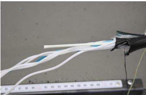
Cut any filling elements at the peeling point and leave the middle element to about 10 cm in length.
