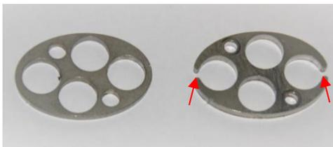
If using XOKO cable glands, dismantle the cable gland and make notches on both sides of the holes in the metal parts.
