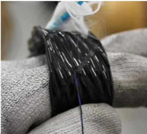
Bend the middle sheath away and find the black and blue tear wire on its inner surface. Remove the end of the tear wire from the sheath with the tip of the knife and pull the wire off the sheath to the split point.
