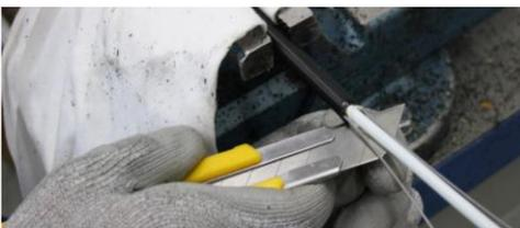
Cut the halves of the sheath and the threads between the sheath and the central tube from the base of the peeling.
