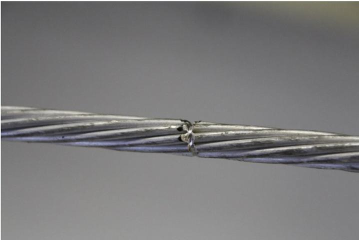
Dismantle the outer layer of wire a few threads at a time and bend them so that they break at the starting point of the peeling.
