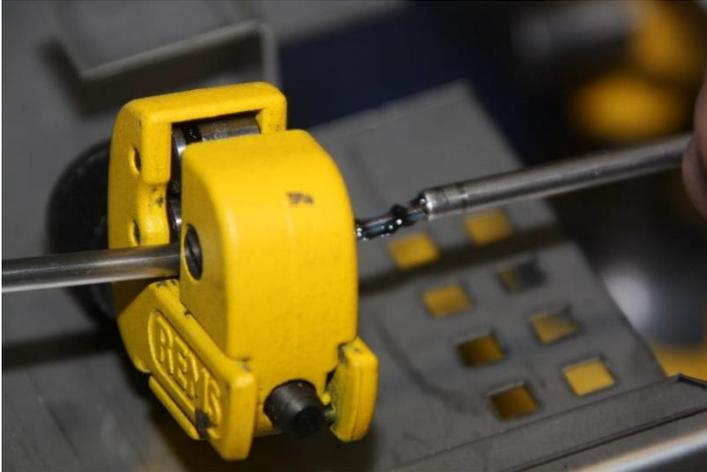
When the fiber tube is broken, remove the tool and gently pull the end of the tube off the fibers, pulling straight ahead.
