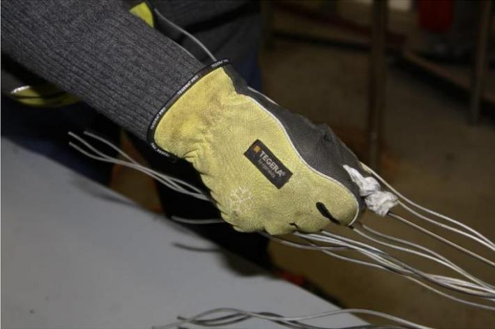
Clean each wire of the inner layer carefully from the grease.
