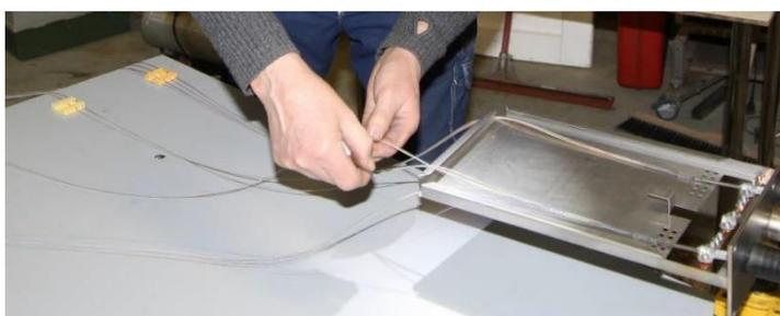
Pull the fibers straight and separate each group of fibers. You can use e.g. splice holders for help.
