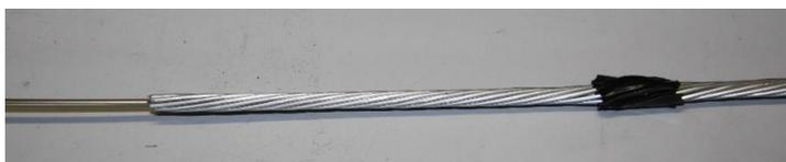
The fiber tube and the inner wire layer is sealed.
