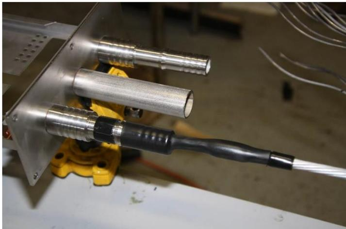
Also install vulcanizing tape at the root of the shrink tube and at the thinned point of the cable pass-through.
