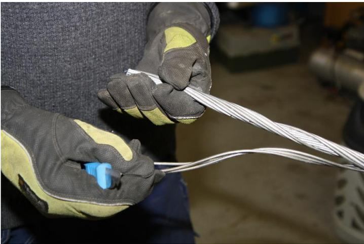
Outer layer of wires removed from the starting point of peeling.
