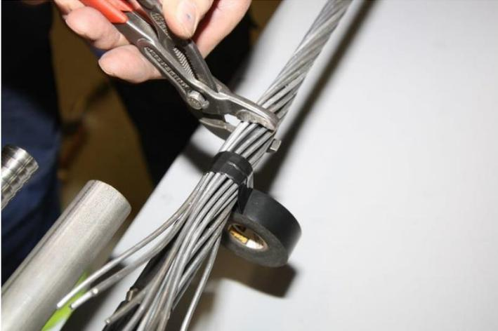
When placing the wires, you can use the help of insulation tape and pliers.
