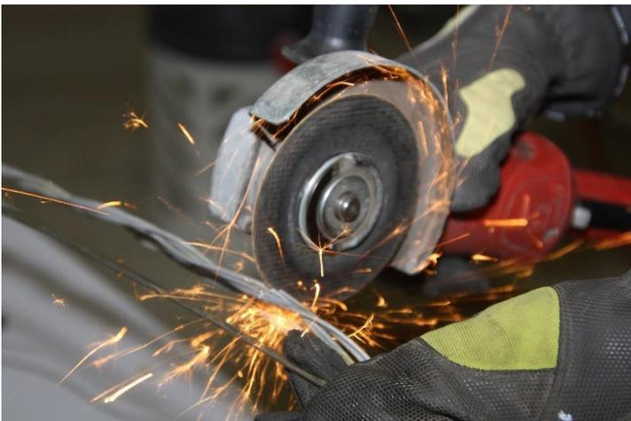
Cut the inner wires from the marked cut-off point, taking care of the steel fiber tubes in the middle of or between the wires.
