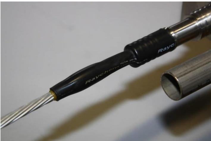
Heat-shrink tube installed
