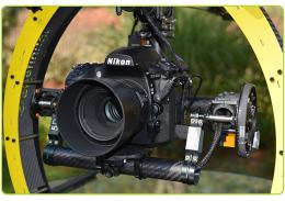
The standard Surveyor 630 UAS includes a Nikon D5300 DSLR outfitted with a 28mm prime lens and GPS.
