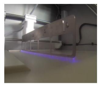
Although ozone is generated as a bi-product of the corona discharge, it is easily eliminated either through existing exhaust systems or through a custom-built Tantec ozone neutralizing system
