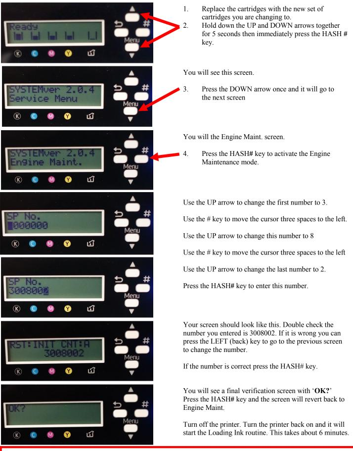
The procedure needs to be repeated once more starting from No.2 (holding down the UP/DOWN keys for 5 seconds). You <u>DO</u> <u>NOT</u> need to replace the set of cartridges you used for the first fill as the new set will comfortably fill the printer twice.
