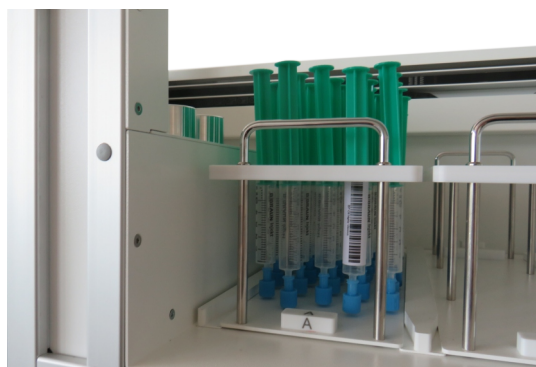
Automatic sample dosing by means of disposable syringes (5 mL)
