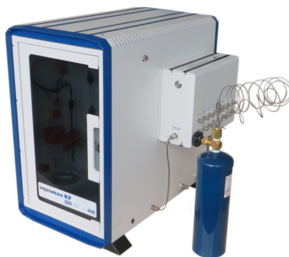
Aquamax KF PRO LPG with connected LPG Selection Box and gas sample cylinder
