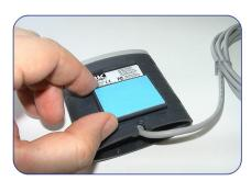
Lift off the pad (reader back) for use without the base.
