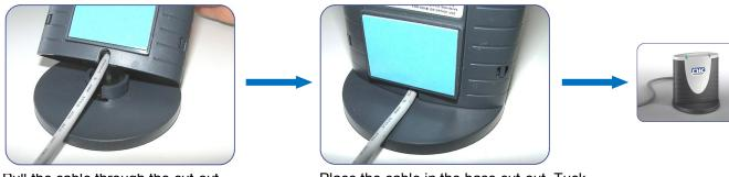
Pull the cable through the cut-out found in the reader back.
